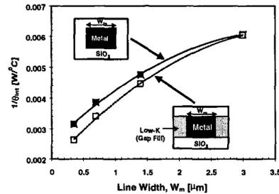
Figure 5. Experimentally obtained effective thermal impedance values for level 1 AlCu metal lines in a  $0.25\text{-}\mu\text{m}$  CMOS process, with two different intra-level dielectrics. The  $t_{ox}$  was  $1.2 \text{ }\mu\text{m}$ , and interconnect length,  $L = 1000 \text{ }\mu\text{m}$ .
