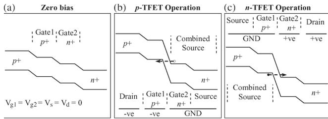
Fig. 5. Band diagrams of the twin-gate TFET at (a) zero bias, (b) p-TFET operation, and (c) n-TFET operation, illustrating the operating principles.
