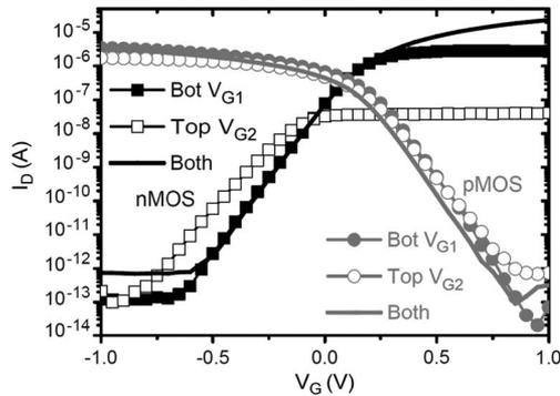
Fig. 3.  $I_D$ - $V_G$  characteristics of the stacked twin-gate n- and p-type transistors measured on 35-nm-diameter silicon nanowires. The drain current is obtained by sweeping  $V_{G1}$  or  $V_{G2}$  while keeping the other one floating, as well as sweeping both  $V_{G1}$  and  $V_{G2}$  together. The drain voltage is kept at  $|1.5|$  V, and the source is grounded.
