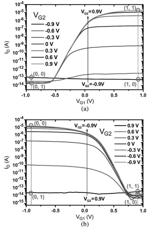
Fig. 4.  $I_D$ - $V_G$  characteristics of the stacked-gate vertical nanowire transistor for (a) nMOS and (b) pMOS measured on 35-nm-diameter Si nanowires. The drain current is obtained by sweeping  $V_{G1}$  for various  $V_{G2}$ . The drain voltage is kept at  $|1.5|$  V, and the source is grounded. The circles indicate four different input states ( $V_{G1}, V_{G2}$ ).
