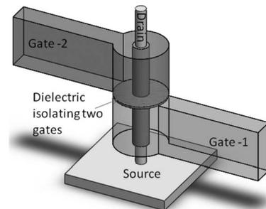
Fig. 1. Schematic showing the 3-D view of the stacked vertical twin-gate nanowire MOSFET.
