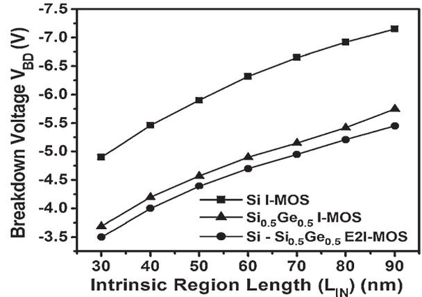
Fig. 3. Comparison of  $V_{BD}$  of n-type Si-Si<sub>0.5</sub>Ge<sub>0.5</sub> E2I-MOS with Si I-MOS and Si<sub>0.5</sub>Ge<sub>0.5</sub> I-MOS at various  $L_{IN}$ 's. E2I-MOS exhibits lower  $V_{BD}$  due to the enhanced electric field near the source.
