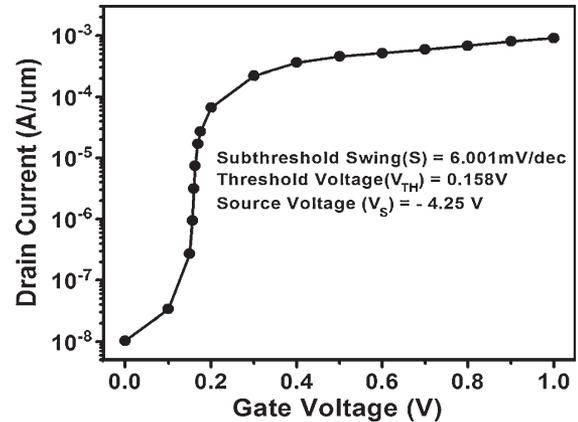
Fig. 4. Simulated  $I_D$ - $V_G$  characteristics of n-type Si-Si<sub>0.5</sub>Ge<sub>0.5</sub> E2I-MOS ( $V_{BD} = -4.4$  V). Subthreshold swing is measured at the inflection point.
