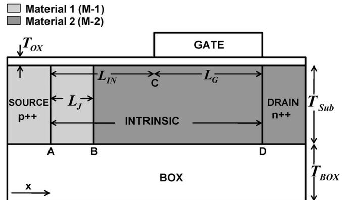
Fig. 1. Basic device structure for n-type E2I-MOS. In all simulations,  $L_G = L_{IN}$  and drain voltage  $V_D = 0$ . Unless mentioned otherwise, the parameters used are as follows:  $L_G = L_{IN} = 50$  nm,  $L_J = 10$  nm,  $T_{OX} = 3$  nm,  $T_{Sub} = 40$  nm,  $T_{BOX} = 350$  nm, gate work function  $\Phi_M = 4.17$  eV, and maximum source/drain doping of  $2 \times 10^{20}$  cm $^{-3}$  with characteristic length of 5 nm.
