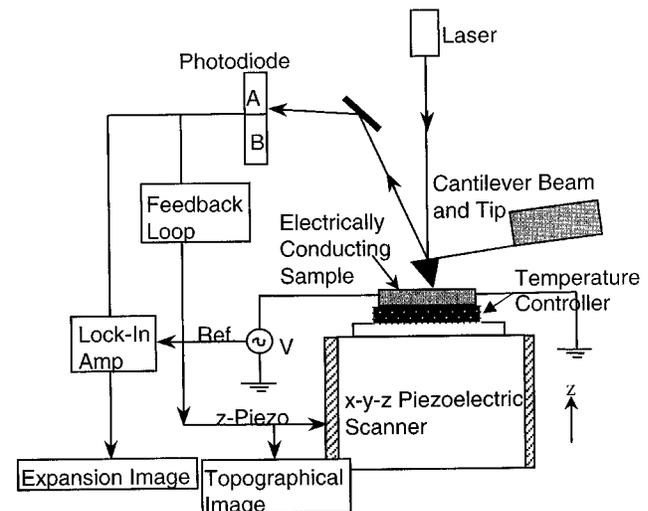
Fig. 1. Schematic diagram of the experimental setup used for the scanning Joule expansion microscopy (SJEM).
