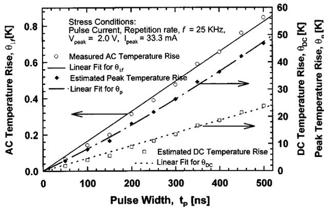
Fig. 4. First harmonic, dc (average) and peak temperature rise on top of the via as a function of the pulsed width of applied pulsed current.
