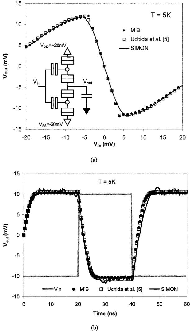
Fig. 3. (a) Static and (b) transient characteristics of an SET inverter cell, as predicted by MIB, SIMON, and Uchida's model [5]. The SET parameters are  $R_S = R_D = 1, \text{M}\Omega$ ,  $C_{TD} = C_{TS} = 1 \text{ aF}$ ,  $C_{G1} = 3 \text{ aF}$ , and the output load capacitor is  $C_L = 1 \text{ fF}$ .
