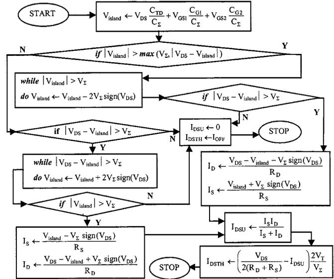
Fig. 1. Simplified flow chart of the computing subroutine  $f$  for SET currents  $I_{DSU}$  and  $I_{DSTH}$ . Here, the  $\text{sign}(V_{DS})$  function holds the sign of  $V_{DS}$ ,  $\max(a, b)$  subroutine returns the maximum between  $a$  and  $b$ ,  $V_T$  is the thermal voltage ( $=kT/e$ ,  $k$  is the Boltzmann's constant),  $V_{\Sigma} = e/(2C_{\Sigma})$ , and  $C_{\Sigma} = C_{TS} + C_{TD} + C_{G1} + C_{G2}$ .
