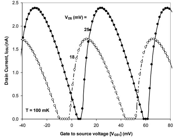
Fig.5.  $I_{DSU}$  model validation for asymmetric SET with:  $C_{G1} = 3\text{aF}$ ,  $R_S = 1\text{M}\Omega$ ,  $R_D = 5\text{M}\Omega$ ,  $C_{TS} = 0.8\text{aF}$ ,  $C_{TD} = 2.2\text{aF}$  where the symbol “●” represents MIB model, the thick line SIMON simulations for a single gate SET. In the same figure “O” represents MIB and dotted line represents SIMON simulations for a *double gate* SET with  $C_{G2} = 1.5\text{aF}$  and  $V_{GS2} = 30\text{mV}$ .
