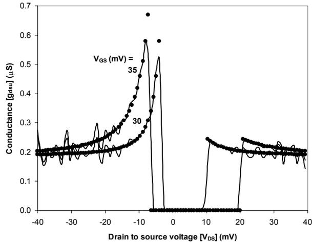
Fig.4. Validation of MIB output conductance model for single gate symmetric device at  $T = 100\text{mK}$  with same parameters and notations as Fig. 2(a).
