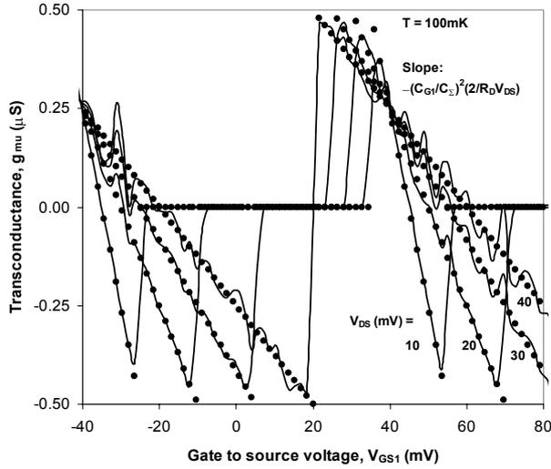
Fig. 3. Validation of MIB transconductance model for single gate symmetric device with same parameters as Fig. 2(a), where the symbol “●” represents MIB model, the thick line denotes the SIMON simulation.
