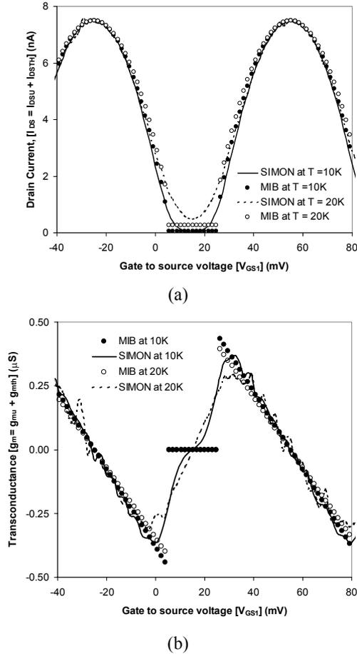
Fig. 6(a) and (b) Validation of MIB drain current and transconductance model at high temperature for single gate SET with the same device parameter as Fig. 2(a).
