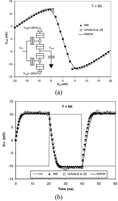
Fig.7(a) and (b). Static (a) and transient (b) characteristics of a SET inverter cell, as predicted by: MIB, SIMON and Uchida's model [6]. The SET parameters are:  $R_S = R_D = 1M\Omega$ ,  $C_{TD} = C_{TS} = 1$  aF,  $C_{G1} = 3$  aF and the output load capacitor is  $C_L = 1f$ .
