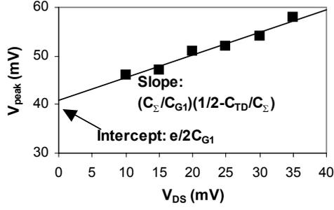
Fig.2(b) linear plot of  $V_{peak}$  versus  $V_{DS}$  for model parameter extraction using a self-consistent validation method. The extraction assumes that  $C_{TD} = C_{TS}$ ,  $I_{peak} \leq e/2C_{\Sigma}(R_D+R_S)$  and corresponds to single-gate SET.
