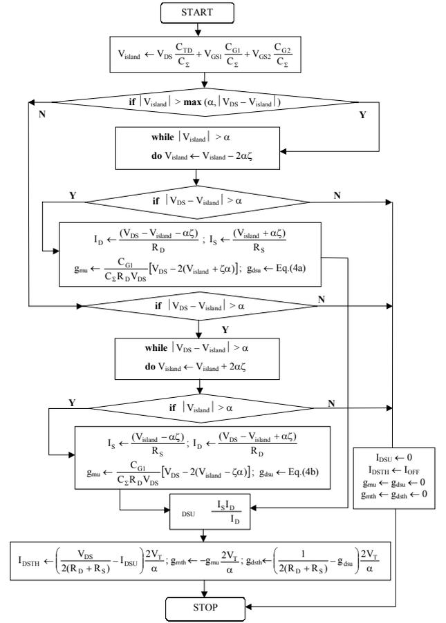
Fig.1. Simplified flow chart of the computing subroutine for SET currents,  $I_{\text{DSU}}$  and  $I_{\text{DSTH}}$ . Here  $\zeta$  function holds the sign of  $V_{\text{DS}}$ ,  $\max(a,b)$  subroutine returns the maximum between a and b,  $V_{\text{T}}$  is the thermal voltage ( $= kT/e$ ,  $k$  is the Boltzmann's constant),  $\alpha = e/(2C_{\Sigma})$ , and  $C_{\Sigma} = C_{\text{G1}} + C_{\text{G2}} + C_{\text{TS}} + C_{\text{TD}}$ .
