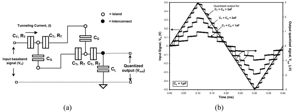
Fig. 3: (a) A SET-based quantizer for hybrid SET-CMOS communications applications [15]:  $C_G$  and  $C_T$  are the gate and tunnel capacitance,  $R_T$  is the tunnel resistance and  $C_L$  is the load capacitance ( $C_L \gg C_G, C_L$ ) and (b) Effect of device capacitance on the sampling rate of the quantizer working at  $T=100mK$ , for three values of device capacitance (1aF, 2aF and 3aF).
