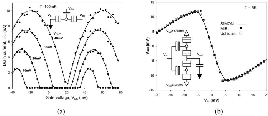
Fig. 2: (a) Periodical, parabolic-shaped,  $I_D$ - $V_{GS}$  characteristics of SET are still able to provide a quasi-conventional behavior of the transfer characteristic of SET inverter (b). Plots are simulated with Monte-Carlo simulator SIMON and also with Uchida [12] and MIB [13] analytical models.
