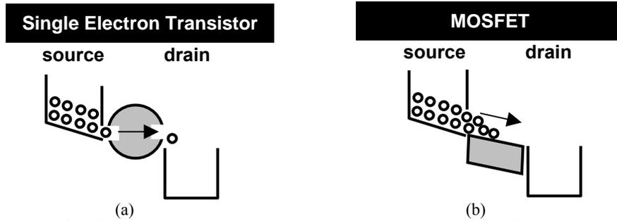
Fig. 1: Transfer of electrons is (a) one-by-one in Single Electron Transistor (SET), which is in contrast with (b) conventional MOSFET where many electrons simultaneously participate to the drain current (after Uchida et al. [11]).
