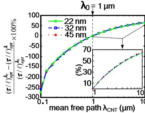
**Fig 7:** Percent improvement in optimal delay per unit length  $(\tau/l)_{opt}$  for buffered CNT bundle global interconnect compared to  $(\tau/l)_{opt}$  for the typical value of  $\lambda_0 = 1 \mu m$ , as  $\lambda_{CNT}$  is varied. Maximum metallic CNT density (dense bundle) is assumed.
