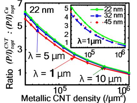
**Fig 8:** Ratio of repeater power dissipation per unit length for optimally buffered CNT-bundle global interconnect to that of Cu, as a function of metallic CNT density and for different mean free path lengths ( $\lambda_{CNT}$ ). Inset: same ratio evaluated at different technology nodes for  $\lambda_{CNT} = 1 \mu m$ .
