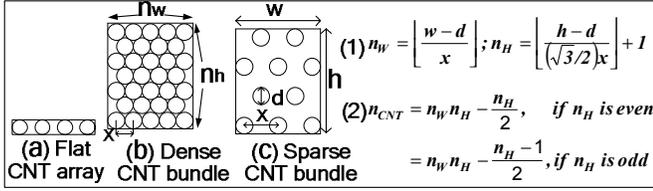
**Fig 1:** Cross-section schematic of CNTs forming (a) flat array, (b) dense bundle ( $x=d$ ) and (c) sparse bundle ( $x>d$ ). Eqs. (1, 2): No. of metallic CNTs ( $n_{CNT}$ ) in bundle, assuming uniform distribution.  $n_w$  and  $n_h$ : number of metallic CNTs along interconnect width and height respectively.
