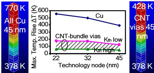
Fig. 12: Maximum interconnect temperature rise for Cu interconnects and vias vs CNT bundle vias integrated with Cu interconnects. For CNT bundles, the shaded region shows the range  $1750$  W/mK  $< K_{th} < 5800$  W/mK [20]. Reference (substrate) temperature = 378 K.
