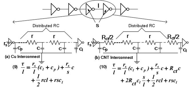
**Fig 5:** Delay per unit length for optimally buffered global interconnects made of (a) Cu and (b) CNT bundle. For CNT interconnects,  $c$  includes  $C_E$  and  $C_Q$  (Fig. 2(b)) and  $r$  is per unit length resistance ( $h/4e^2$ )/ $\lambda_{CNT}$ .
