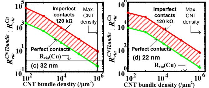
Fig 13: (a) Via dimensions at 45 nm node (via height  $< \lambda_{CNT}$ ). (b-d) Ratio of CNT bundle via resistance to Cu via resistance as a function of CNT bundle density, at (b) 45 nm, (c) 32 nm, (d) 22 nm nodes. Shaded region: imperfect metal-nanotube contact resistance  $0 < R_{ct} < 120$  K $\Omega$  [10].
