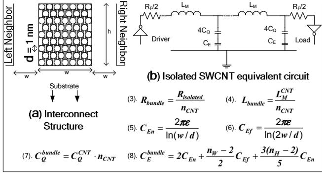
**Fig 2:** (a) Interconnect structure and (b) Equivalent circuit [12] for isolated SWCNT. Equations 3-8: equivalent circuit parameters for a CNT bundle interconnect.  $C_{En}$  and  $C_{Ef}$  are parallel plate capacitances of isolated CNT with respect to near and far neighboring interconnects respectively [17].
