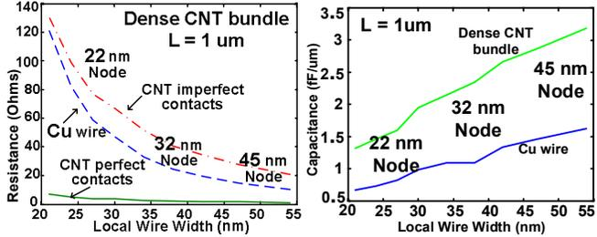
**Fig 3:** (a) Resistance and (b) Capacitance of  $1 \mu m$  long local interconnect using densely packed CNT bundles compared with Cu at different technology nodes (assuming  $\lambda_{CNT} = 1 \mu m$  [3]).
