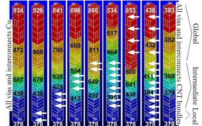
Fig 15: Interconnect temperature contour plots showing interconnect temperature (K) at different layers from 3D finite element electrothermal simulations (22 nm node). Leftmost: all interconnects and vias are Cu. Rightmost: all interconnects and vias are CNT bundles. In remaining images, each arrow points to a particular interconnect level where the vias are assumed to be composed of CNT bundles, while all other vias and all interconnects are made of Cu.
