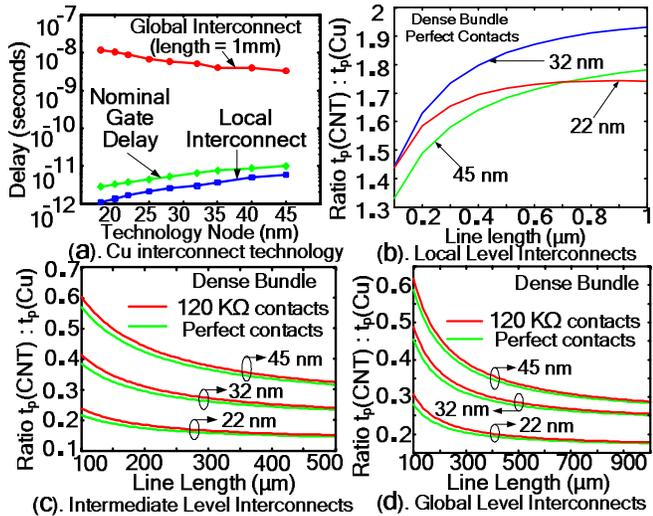
**Fig 4:** (a) Typical delay for global and local Cu interconnects compared to nominal gate delay [18], as technology scales. (b-d) Ratio of CNT interconnect delay (assuming  $\lambda_{CNT} = 1 \mu m$  [3]) to that of Cu interconnect of same dimensions at (b) local, (c) intermediate and (d) global levels.
