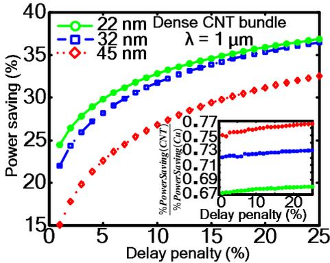
Fig. 10: Percent saving in repeater power dissipation per unit length for “power-optimal” buffer inserted CNT-bundle global interconnect as a function of delay penalty (% of  $(\tau/l)_{opt}$ ). Inset: Ratio of % power saving with CNT bundle to that with Cu.
