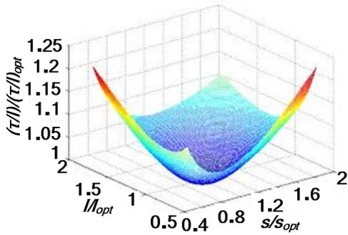
Fig 9: Delay per unit length in sub-optimally buffered CNT bundle global interconnect normalized to optimal delay per unit length, as a function of sub-optimal repeater size ( $s$ ) and inter-repeater separation ( $l$ ).
