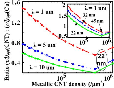
**Fig 6:** Ratio of optimal delay per unit length for buffered CNT bundle global interconnect to that of Cu, as a function of density of metallic CNTs in the bundle: for different mean free paths ( $\lambda$ ) at 22 nm node (main fig.) and at different technology nodes (inset).
