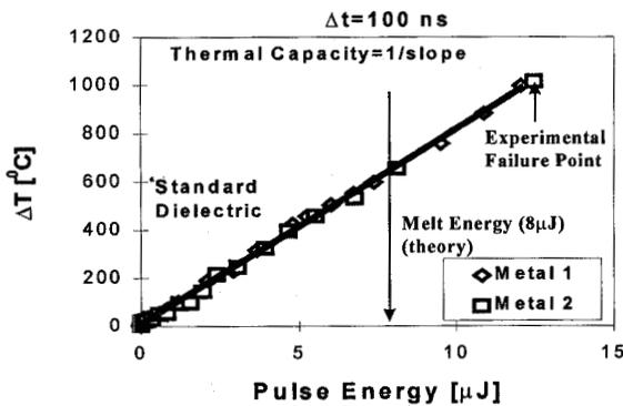
Figure 5. The thermal capacity of (3 μm) metal 1 and metal 2 is identical in case of the standard dielectric process in agreement with Fig. 4.
