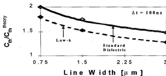
Figure 14. Ratio of experimental and theoretical thermal capacities increases with scaling due to increasing heat conduction into the oxide sheath.
