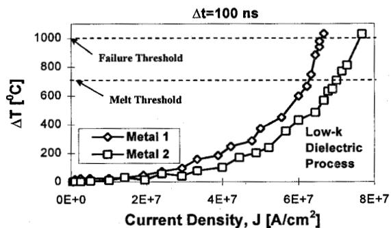
Figure 6. Self heating and failure for 3 μm X 1000 μm metal lines for a 100 ns pulse with metal 1 embedded in low-k along the sides (gap fill).
