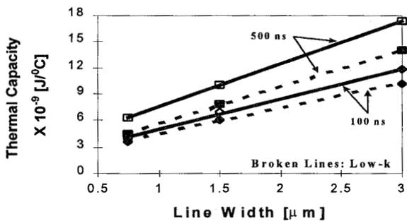
Figure 13. Thermal capacity variation with interconnect scaling and the effect of low-k dielectric for various pulse widths. The relative effect of low-k on the thermal capacities is larger for narrower metal leads and wider pulse widths.
