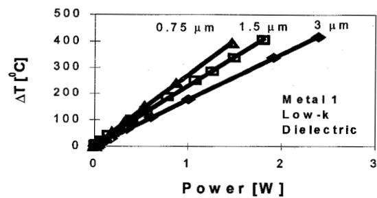
Figure 2. DC self heating effect of metal 1 lines with the low-k dielectric is more severe.
