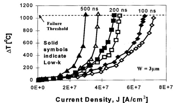
Figure 8. Effect of low-k dielectric on the critical current density in 3 μm X 1000 μm metal 1 leads summarized for various pulse widths.
