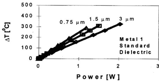
Figure 1. Effect of interconnect scaling on the DC self heating of metal 1 lines with the standard dielectric.
