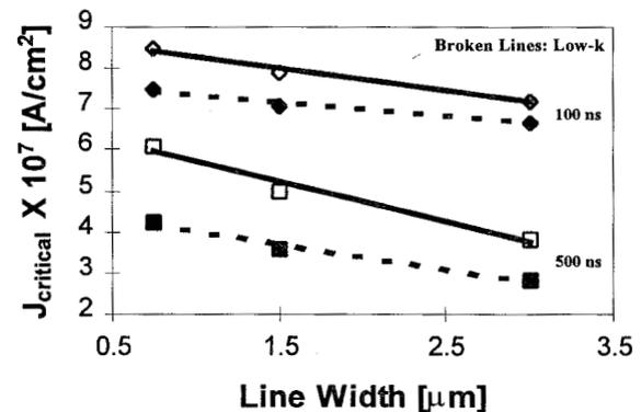
Figure 15. Effect of interconnect scaling and low-k dielectric on the critical current density for metal 1 leads stressed by current pulses of varying widths.  $J_{critical}$  increases for decreasing line width as shown in Fig.12. The effect of low-k lowers the critical values further. As line widths gets smaller and pulse widths get larger the effect of low-k gets even worse.
