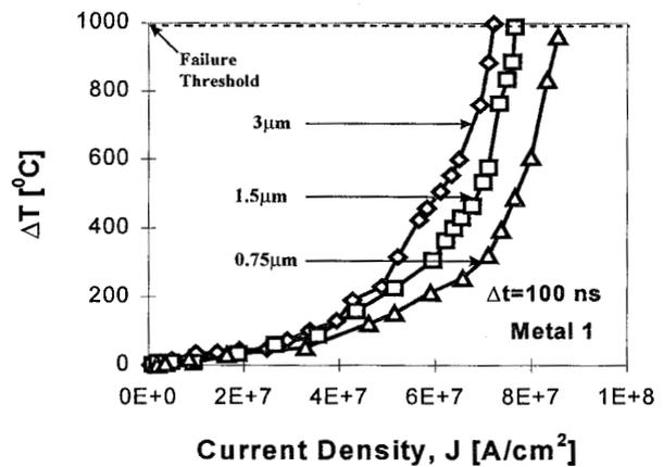
Figure 12. Effect of line width reduction on metal heating. The wider lines heat up more rapidly owing to their smaller surface area to volume ratio (for metal 1 standard dielectric process).
