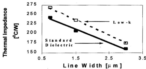
Figure 3. Thermal impedance of metal 1 is higher for the low-k dielectric and increases further as line width decreases.
