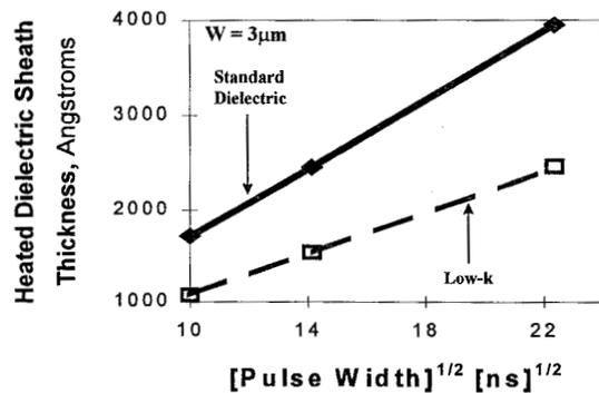
Figure 10. Thickness of the heated dielectric sheath is lower for the low-k material, which results in their lower thermal capacities as shown in Figure 9.
