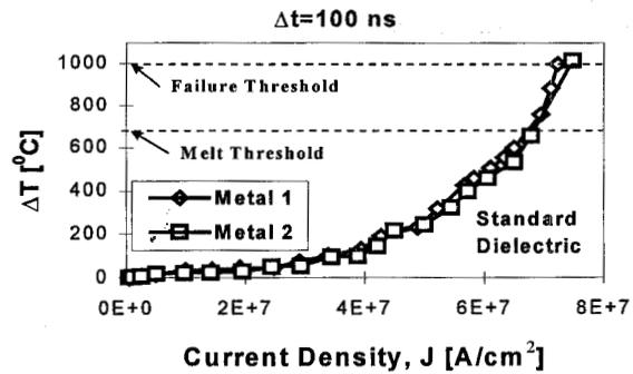
Figure 4. Self heating and failure for 3 μm X 1000 μm metal lines for a 100 ns pulse shown for the standard dielectric process.
