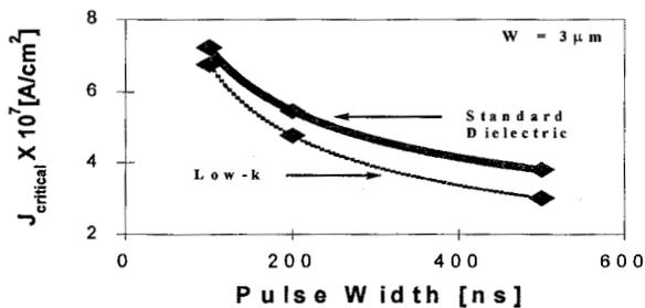
Figure 11. Critical current density of metal 1 leads decreases with increasing pulse width. For the low-k structures,  $J_{critical}$  is further lowered by about 10%.
