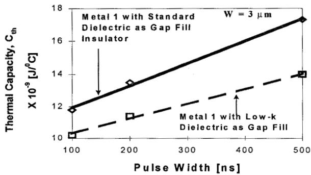
Figure 9. Thermal capacity increases with pulse width and is relatively lower for the low-k embedded metal.
