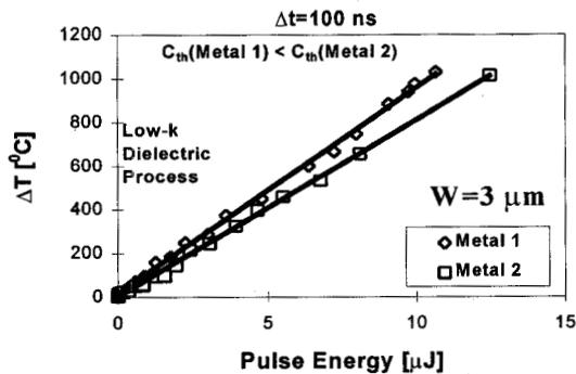
Figure 7. Thermal capacity ( $C_{th}=1/slope$ ) of metal 1 is less than that of metal 2. Metal 1 with low-k requires  $\sim 7\mu J$  and metal 2 without low-k requires  $\sim 9\mu J$  to reach the melt temperature of  $\sim 660^\circ C$ .
