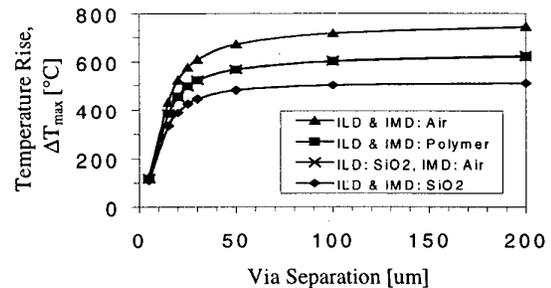
Figure 8.  $\Delta T_{max}$  of global interconnects for a 200 ns current pulse with  $J=6 \times 10^7$  A/cm<sup>2</sup>.  $\Delta T_{max}$  increases with via separation and saturates when via effect has diminished.
