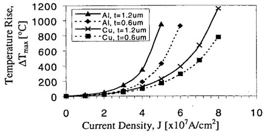
Figure 5. For the same wire cross section, shown in Fig. 3, Cu wire shows much lower temperature rise compared to Al wire under a 200 ns pulse stress. Symbols represent simulation points.
