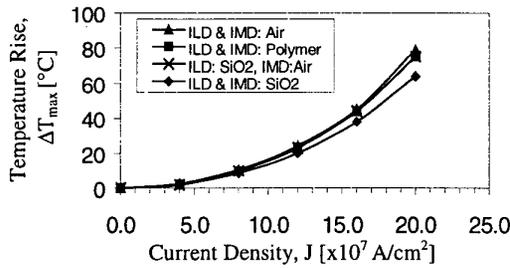
Figure 11.  $\Delta T_{max}$  of Cu local interconnect with 1  $\mu\text{m}$  via separation under a 200 ns current pulse. Temperature rises are much lower and nearly independent of the surrounding dielectric materials.
