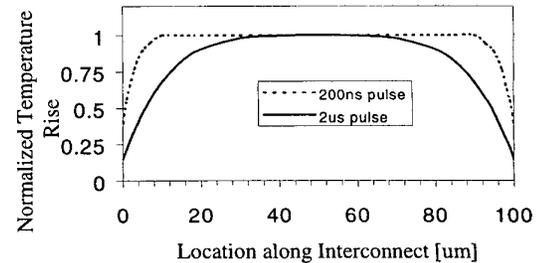
Figure 6. Simulated normalized temperature ( $\Delta T/\Delta T_{max}$ ) profile along global Cu interconnect for two pulse durations with current density  $J=4 \times 10^7$  A/cm<sup>2</sup>.
