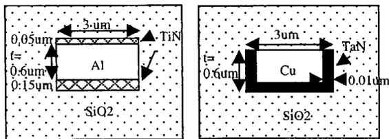
Figure 3. Schematic cross section of Al and Cu interconnects with cladding layers used in model validation Fig. 4 and for simulations in Fig. 5.
