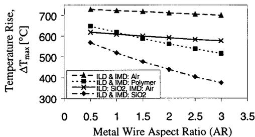
Figure 15. For the same metal thickness (2.5  $\mu\text{m}$ ), global interconnects with lower AR, shows higher  $\Delta T_{max}$  due to lower surface area-to-volume ratio.  $t_{pulse} = 200 \text{ ns}$  and  $J=6 \times 10^7 \text{ A/cm}^2$ .
