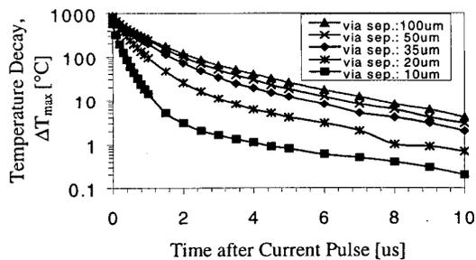
Figure 7. The temperature decay after a 200 ns current pulse, for Cu/low-k (polymer) global wires. The decay is facilitated by the presence of vias.
