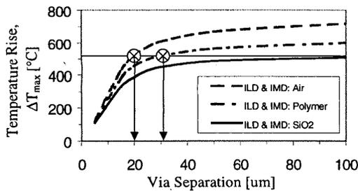
Figure 13.  $\Delta T_{max}$  of Cu/air and Cu/polymer can match  $\Delta T_{max}$  of Cu/oxide global interconnect if dummy thermal vias are added every 20  $\mu\text{m}$  and 30  $\mu\text{m}$ , respectively, with  $t_{pulse} = 200 \text{ ns}$  and  $J=6 \times 10^7 \text{ A/cm}^2$ .
