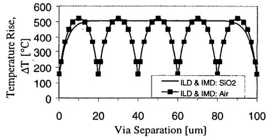
Figure 14. Cu/air with thermal vias every 20  $\mu\text{m}$  shows nearly the same  $\Delta T_{max}$  as that of Cu/oxide global interconnect with 100  $\mu\text{m}$  via separation under a 200 ns and  $J=6 \times 10^7 \text{ A/cm}^2$  current pulse.
