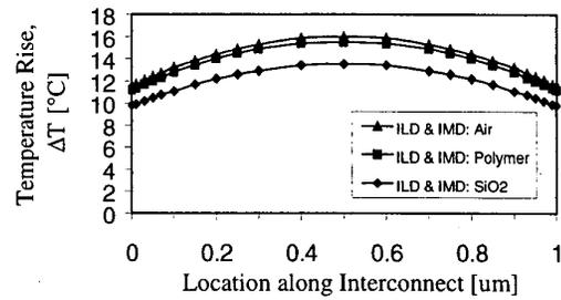
Figure 12. Temperature profiles along local Cu interconnect under a 200 ns pulse are gradual for all the dielectric materials and  $\Delta T_{max}$  are about the same with  $J=1 \times 10^8 \text{ A/cm}^2$ .
