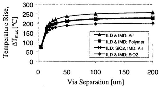
Figure 9. For a short pulse of 100 ns, with the same current density as in Fig. 8,  $\Delta T_{max}$  of the global Cu interconnect is much less dependent on the dielectric materials.
