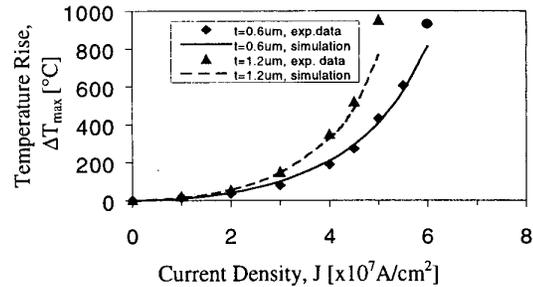
Figure 4. Validation of HSPICE thermal simulation with experimental data from [10]. Al interconnect test structure shown in Fig. 3 is used.
