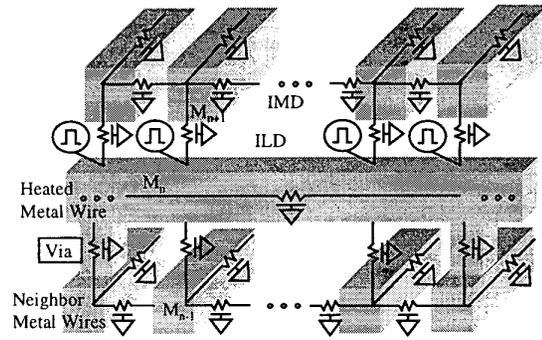
Figure 2. 3-D thermal circuit RC transmission line model for transient thermal analysis of interconnect structures.
