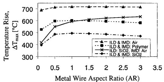
Figure 16. For the same metal wire cross section area (5  $\mu\text{m}^2$ ), the impact of AR and dielectric structure strategy is shown.  $\Delta T_{max}$  peaks at AR=1 due to the smallest perimeters.  $t_{pulse} = 200 \text{ ns}$  and  $J=6 \times 10^7 \text{ A/cm}^2$ .
