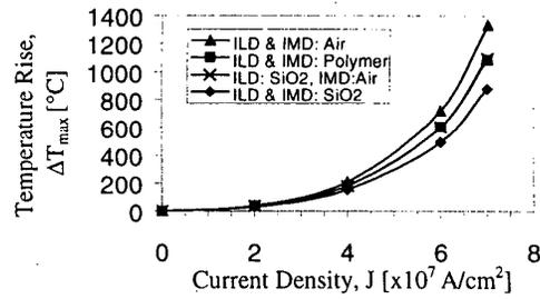
Figure 10.  $\Delta T_{max}$  of Cu global interconnect with 100  $\mu\text{m}$  via separation under a 200 ns current pulse. Temperature rises sharply with current density.
