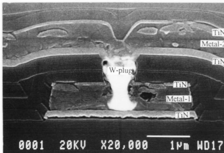
**Figure 7.** SEM micrograph showing the displaced W-plug (the early time-to-failure unit). The e-flow direction was from metal 2 to metal 1. Al voiding is evident in metal 1.
