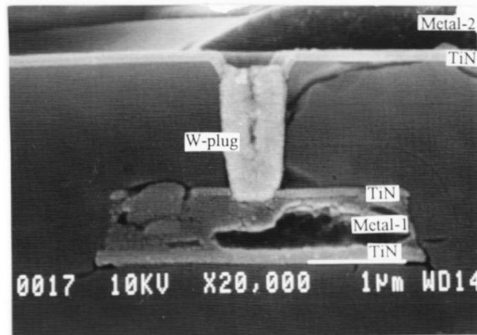
**Figure 11.** SEM micrograph showing void formation at the bottom of via with Ti/TiN cap. The e-flow direction was from metal 2 to metal 1. A worst-case aspect ratio of 3:1 was used for this particular evaluation. Aluminium voiding is evident in metal 1.
