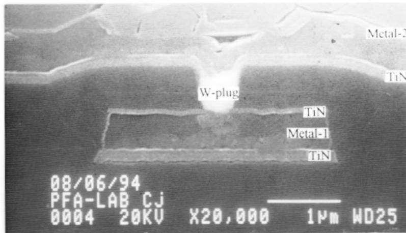
**Figure 9.** SEM micrograph showing the late time-to-failure unit. The e-flow direction was from metal 2 to metal 1. An accumulation of aluminium in metal 2 (over the via) is evident causing interlevel oxide cracking.
