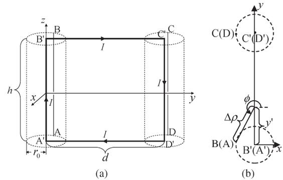
Fig. 5. Schematic overview of two TSVs showing various geometrical parameters used in (11)–(25): (a) the entire view of the structure and (b) the top view.
