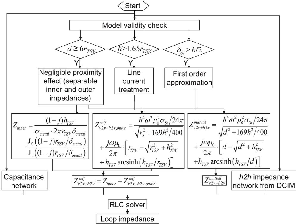
Fig. 11. Flowchart of loop impedance extraction with both TSVs and horizontal interconnects in 3-D IC.
