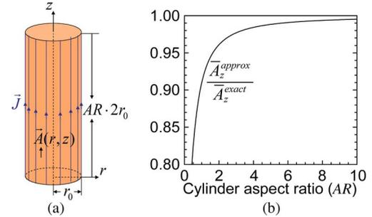
Fig. 4. (a) From a cylinder carrying a uniform  $z$ -directional current  $J_z$  at the outskirts, one can examine the average  $z$ -directional vector potential at the outskirts of a cylinder in free space, the value of which can be obtained either from an exact method or from an approximate method that treats the current as a line current at the center of the cylinder. (b) Ratio of the value from the approximate method to that from the exact method.
