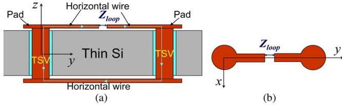
Fig. 3. (a) Cross-sectional view and (b) top view of a TSV horizontal wire loop (without consideration of the lower substrate).
