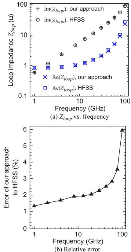
Fig. 10. (a) Loop impedance  $Z_{loop}$  of the structure shown in Fig. 9(a) from both our approach and HFSS [20]; (b) relative error of our approach against the HFSS result (the definition of the relative error is the same as in Fig. 8).
