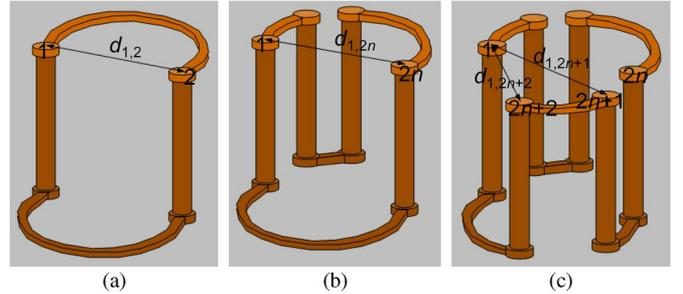
Fig. 12. Schematic figures during the mathematical induction proof; as we prove (a) the most simple case (wire loop with two TSVs and two horizontal wires) and the recurrence relation from (b) the case of wire loop with  $2n$  TSVs and  $2n$  horizontal wires to (c) the case of wire loop with  $2n+2$  TSVs and  $2n+2$  horizontal wires, we demonstrate that combining v2v and h2v loop outer series impedances [see (24) and (25)] is valid for any wire loop.
