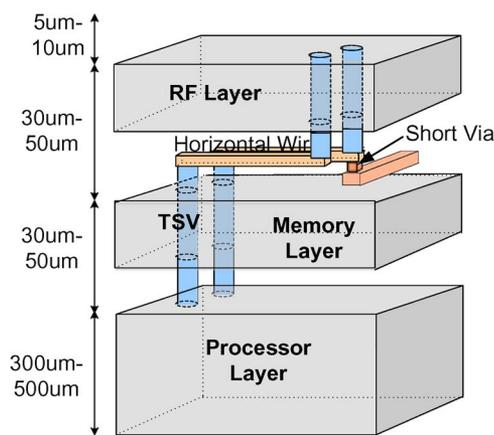
Fig. 1. Schematic view of a 3-D IC.
