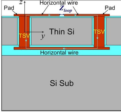
Fig. 2. Cross-sectional view of a TSV horizontal wire loop.
