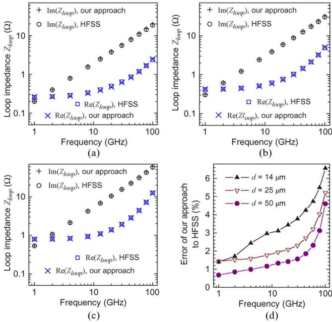
Fig. 8. Loop impedance  $Z_{loop}$  of the structure shown in Fig. 7(a) from both our approach and HFSS [20] with various c2c distances  $d$  between TSVs: (a)  $d = 14 \mu\text{m}$ ; (b)  $d = 25 \mu\text{m}$ ; and (c)  $d = 50 \mu\text{m}$ . (d) Relative error of our approach against the HFSS result with various  $d$ 's, where the relative error is defined as  $|Z_{loop}^{our\ approach} - Z_{loop}^{HFSS}| / |Z_{loop}^{HFSS}|$ .
