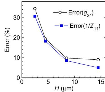
Fig. 1. Calculation error of our analytical model for  $1/Z_{11}$  and  $g_{21}$  at 10 GHz. All the geometrical and material parameters are kept the same as those in [1, Fig. 6], except that we vary the substrate height  $H$  (see [1, Fig. 1(a)]).
