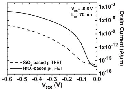
Fig. 11. Input transfer characteristics of vertical p-T-FET, using  $\text{SiO}_2$  with  $x = 0.3$  and  $\text{HfO}_2$  with  $x = 0.3$ . The high- $k$  material gives better  $I_{ON}$ ,  $S$ , and  $V_{th}$ . Using high- $k$  material, the magnitude of  $V_{th}$  is reduced from 0.54 to 0.22 V, and  $S$  is reduced from 50 to 22 mV/dec. Gate-oxide thickness is 1.5 nm for  $\text{SiO}_2$  and 2.5 nm for  $\text{HfO}_2$ .
