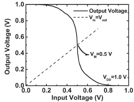
Fig. 14. VTC curve for the T-FET-based inverter. Gain is equal to 12 V/V in the transition region. By employing bandgap and workfunction engineering, both n- and p-type devices were designed to exhibit similar input/output characteristics.
