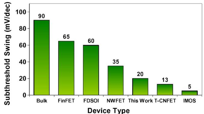
Fig. 1. Subthreshold swings ( $S$ ) reported for various CMOS and emerging solid-state devices. CMOS devices show  $S \geq 60 \text{ mV}/\text{dec}$ . The proposed T-FETs, T-CNFET, and IMOS devices exhibit the smallest values of  $S$ .
