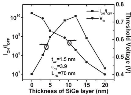
Fig. 10.  $I_{ON}/I_{OFF}$  ratio and threshold voltage of  $\text{SiO}_2$ -based p-T-FET versus thickness of SiGe layer. The threshold voltage decreases as the thickness increases, but the  $I_{ON}/I_{OFF}$  ratio reaches its maximum value with a SiGe layer of 12 nm width.
