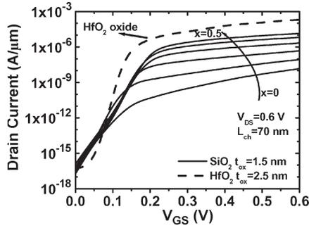
Fig. 5. Transfer characteristics of the vertical n-T-FET, for (dashed line) HfO<sub>2</sub> at  $x = 0.5$  and for (solid line) SiO<sub>2</sub> for  $x = 0.0$  to  $x = 0.5$ ;  $x$  is mole fraction of Ge in SiGe layer. Increasing  $x$  results in higher  $I_{ON}$  and lower  $S$ , with small effect on  $I_{OFF}$ .
