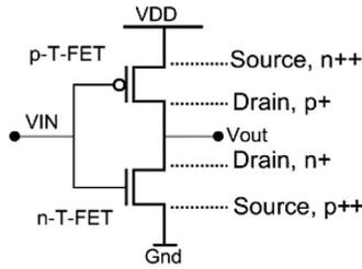
Fig. 12. Inverter-circuit schematic using T-FETs. Both T-FETs must be in reverse-biased region. Unlike MOSFETs, the T-FET device is not a symmetric device, and special care is needed when designing circuits to avoid forward-biased p-i-n structures. Tunneling happens near the source region for both T-FETs.
