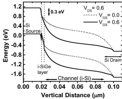
Fig. 2. Band profile for the proposed n-T-FET for different gate voltages. By applying sufficient gate voltage, current flows due to quantum tunneling of carriers. The intrinsic SiGe layer leads to improved  $S$  and  $I_{ON}$ . By taking advantage of the small bandgap of SiGe, a lower gate voltage is required to bend the bands compared with the Silicon-based devices. Intrinsic doping of SiGe layer allows bending of the bands in this layer, resulting in higher ON current.
