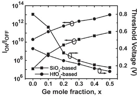
Fig. 8. (Left  $y$ -axis)  $I_{ON}/I_{OFF}$  ratio and (right  $y$ -axis) threshold voltage for high- $k$ -based and  $\text{SiO}_2$ -based n-T-FET devices as a function of Ge mole fraction  $x$ . A higher value of  $x$  improves the performance of both devices.
