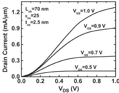
Fig. 13. Output transfer characteristics of vertical n-T-FET, using high-*k* gate oxide with  $x = 0.5$ . Like MOSFET, saturation behavior is observed.
