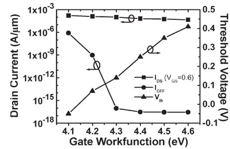
Fig. 7. Effect of gate workfunction on the performance of high- $k$  gate-oxide-based n-T-FET.  $I_{OFF}$  is measured at  $V_{GS} = 0$  V, and  $I_{DS}$  is measured at  $V_{GS} = 0.6$  V and  $V_{DS} = 0.6$ .
