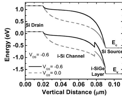
Fig. 9. Band profile of  $\text{SiO}_2$ -based p-T-FET for different values of gate voltage. Using a 10-nm SiGe layer and workfunction engineering, the bands are bent at  $V_{GS} = -0.6$ , allowing tunneling current to flow. By increasing  $V_{GS}$ , the current will decrease.
