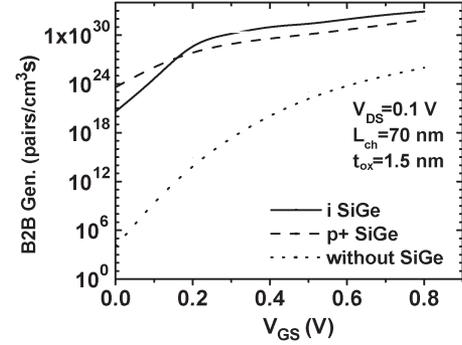
Fig. 6. B2B generation rate ( $G_{B2B}$ ) of n-T-FET for 1) intrinsic SiGe layer, 2) heavily doped SiGe layer [12] and 3) without SiGe layer. The proposed device with undoped SiGe layer shows higher  $G_{B2B}$  at high  $V_{GS}$  and low  $G_{B2B}$  at low  $V_{GS}$ , resulting in better ON current and lower OFF current.
