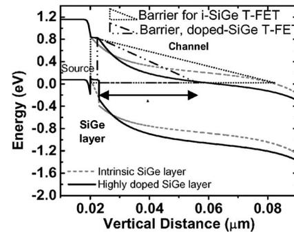
Fig. 4. Approximating the B2B tunneling barrier with a triangular potential barrier for i-SiGe-based T-FET and doped-SiGe-based T-FET at  $V_{DS} = 0.6 \text{ V}$  and  $V_{GS} = 0.0 \text{ V}$  (OFF state for both devices). The i-SiGe-based device has a larger tunneling barrier and shows lower OFF current compared with the highly doped-SiGe-based T-FET. At  $V_{GS} = 0.6$ , the i-SiGe-based device has higher ON current due to band bending in the SiGe layer.
