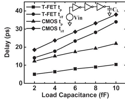
Fig. 15. Comparison of delay for LP CMOS and the proposed T-FET-based inverters. Propagation delay ( $t_p$ ) and rise/fall time ( $t_{r/f}$ ) for the inverter driving  $C_L$  are measured for different values of external load capacitance.
