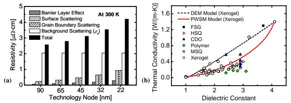
**Fig. 1:** (a) Scaling of metal resistivity for the ITRS intermediate tier wires (at 300K) [3]. (b) Correlation of the thermal conductivity and dielectric constant of ILDs. Inter-layer dielectric constant is lowered as technology scales (for improvement in performance), but thermal conductivity of the dielectric also decreases rapidly [3].
