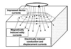
**Fig. 7:** Schematic representation of magnetically induced substrate eddy currents [11].
