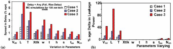
**Fig. 9:** Percentage spread in buffered global interconnect delay and leakage power dissipation for different percentage variations (Case 1: 10%, Case 2: 20%, Case 3: 30%) in different parameters ( $V_{dd}$ : supply voltage, L: channel length, T: temperature, Xtlk: interconnect crosstalk, w: interconnect width, t: interconnect thickness, h: inter-layer dielectric thickness, s: wire spacing,  $t_{ox}$ : gate oxide thickness and  $N_{ch}$ : doping concentration) [19].
