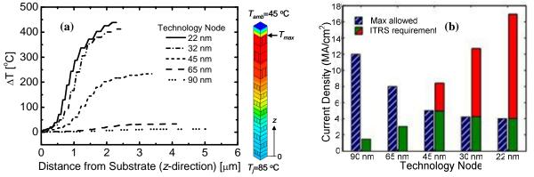
**Fig. 2.** (a) Temperature rise  $(\Delta T)$  along the vertical distance from the substrate at different technology nodes [3]. The temperature contour plot of 45 nm technology node is also shown as an example. (b) Maximum allowed current density (duty ratio=0.001) in local vias from self-consistent electromigration lifetime estimation [5] vs. the ITRS requirement for current density.
