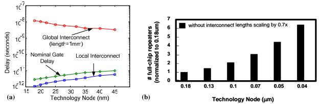
**Fig. 3: (a)** Typical delay for global and local Cu interconnects compared to nominal gate delay [1], as technology scales. (b) Number of repeaters increases rapidly with technology scaling [courtesy of Intel].
