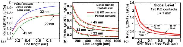
Figure 11: Ratio of interconnect propagation delay with CNT bundle interconnect to that with Cu wire of same dimensions for (a) local interconnect and (b) global interconnect, as a function of interconnect length, and (c) for global interconnect as a function of CNT mean free path [27].
