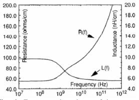
**Fig. 6:** Frequency dependence of interconnect resistance and inductance as a result of skin and proximity effects [8].
