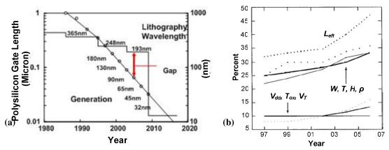
**Fig. 8:** (a) Increasing gap between polysilicon gate length and lithographic wavelength for different technology nodes [15]. (b) Percent variations in device ( $V_{dd}$ ,  $T_{ox}$ ,  $V_T$  and  $L_{eff}$ ) and interconnect (W, T, H,  $\rho$ ) parameters as technology scales [16].
