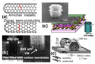
**Figure 10:** (a) Different configurations and resulting electrical conduction types of carbon nanotubes depending on the direction along which the graphene sheets are rolled up (chirality) [23]. (b-d) Strategies to form interconnects and vias using carbon nanotube bundles (b: [24], c: [25], d: [26]).
