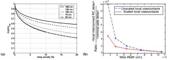
**Fig. 4: (a)** Normalized power per unit length for a buffered global interconnect (normalized to power per unit length for optimally buffered case) as a function of delay penalty [6]. (b) Ratio of local interconnect RC delay (including 2 contacts + 2 local vias) to nominal gate delay as per ITRS, as technology scales [4].
