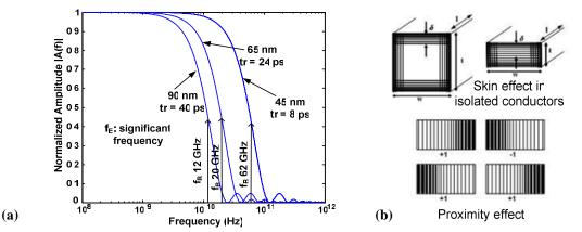
**Fig. 5:** (a) Frequency components of a digital VLSI signal at different technology nodes. The signal rise time (obtained from SPICE simulations) and significant frequency at each technology node are also shown. (b) Schematic depicting current density distribution under skin and proximity effects.
