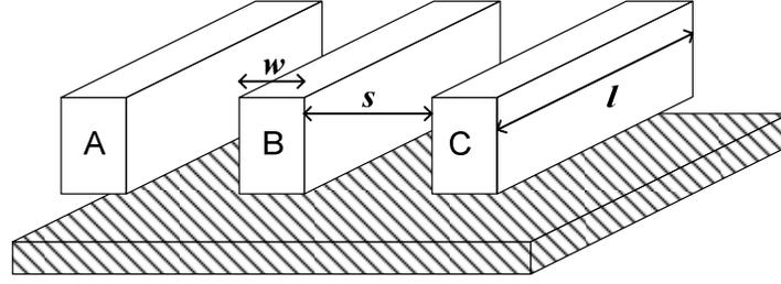
**Figure 1: Interconnect schematic showing parameters for capacitance modeling. In 2D, the capacitance between conductors B and C is independent of the conductor A.**
