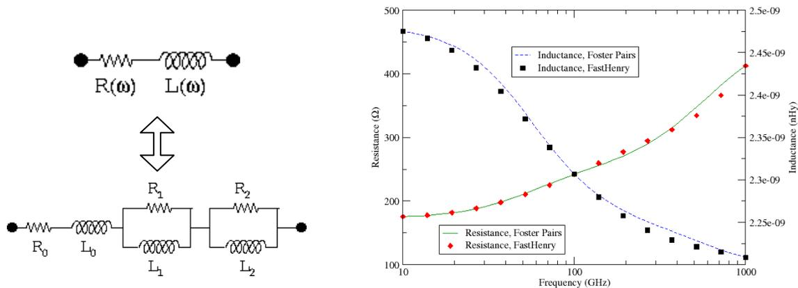
Figure 4: Foster pair representation of frequency dependant RL circuit. The figure at the left shows a typical Foster pair configuration. The plots at the right compare the output of this representative circuit (lines) against FastHenry (symbols).
