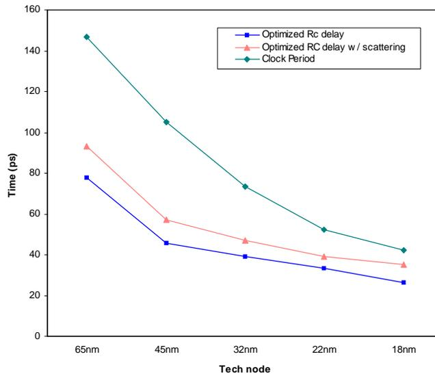
**Figure 8: RC delay (with and without scattering effects) for a 3 mm long optimally buffered global interconnect with scaled wires. The clock period at each technology node is shown for comparison.**
