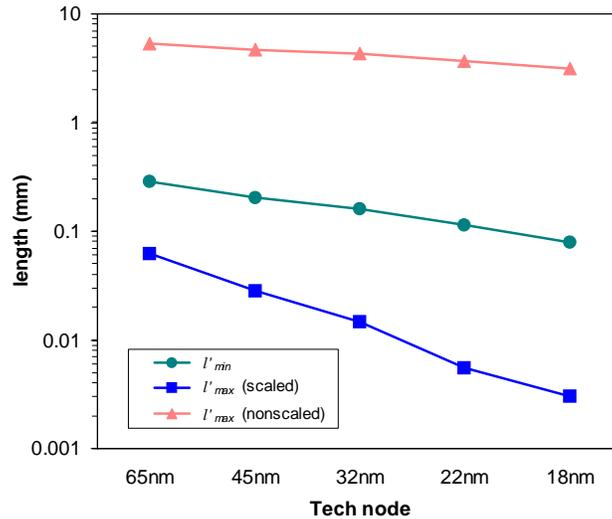
Figure 10: Length restrictions on global wires for RLC transmission.
