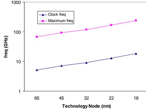
Figure 5: Maximum frequency (corresponding to one FO4 delay) and maximum clock frequency (13 FO4 delays) for a given technology node.
