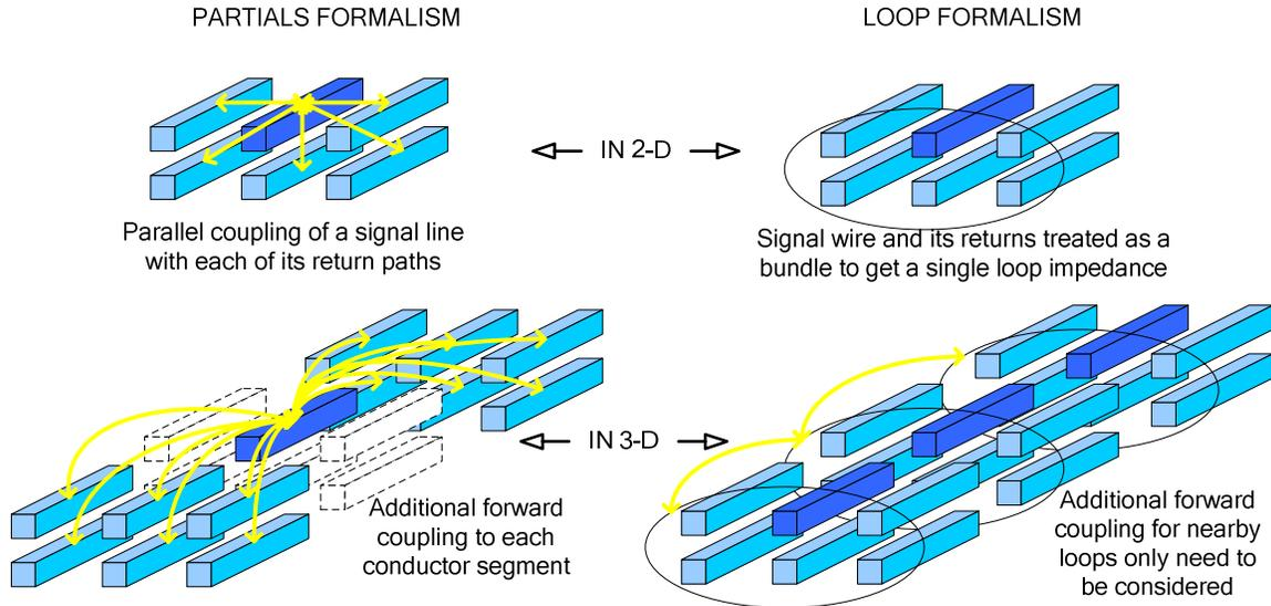
Figure 3: Schematic comparing the partials (PEEC) and loop impedance approaches to inductance extraction, in 2D as well as with corrections due to forward couplings in 3D.
