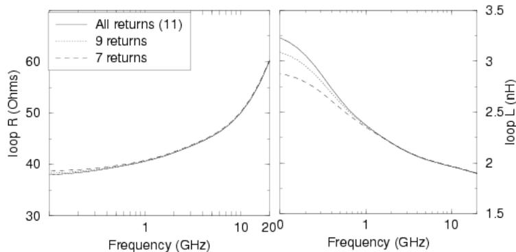
**Figure 2: Loop Impedance (resistance and inductance) of 1 signal wire plus 9 closest ground return paths, separate and total contribution. Wire transverse dimensions are unscaled 1 micron widths.**
