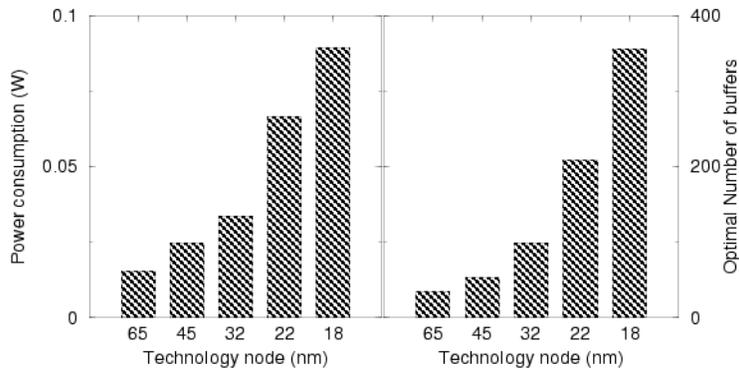
**Figure 9: Number of repeaters and their power consumption for optimal delay on a 3 mm scaled RC line ( $w=3\lambda$ ).**
