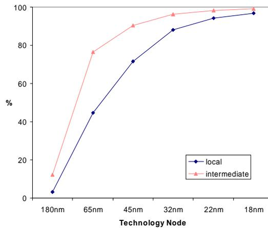
Figure 6: Percentage of RC wire delay influenced by wire resistance.
