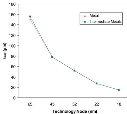
Figure 7: Length limits for local and intermediate wires with maximum noise of  $V_n/V_{dd} = 0.25$ .
